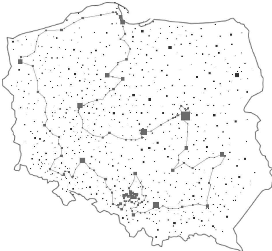
**Fig. 1.** The best path found for a network of Poland ( $C_{max} = 3000$  km). The route starts and ends in Warsaw, it's length is 2999.81 km and profit is 14966 (almost 15 million of inhabitants in visited cities).
